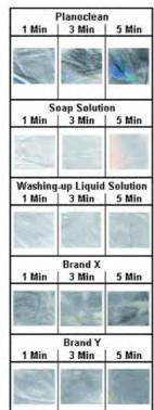
Siemens Industrial Turbomachinery AB conducted a product test. Planoclean<sup>™</sup> was compared with two competing brands and solutions of soap and washing-up liquid.
